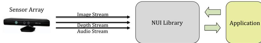
Figure 1. Interaction between the Kinect software and hardware [4].
